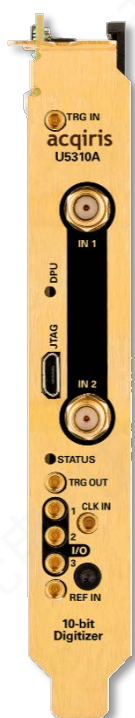
Figure 3. U5310A front panel with analog inputs and multiple I/Os signals.
