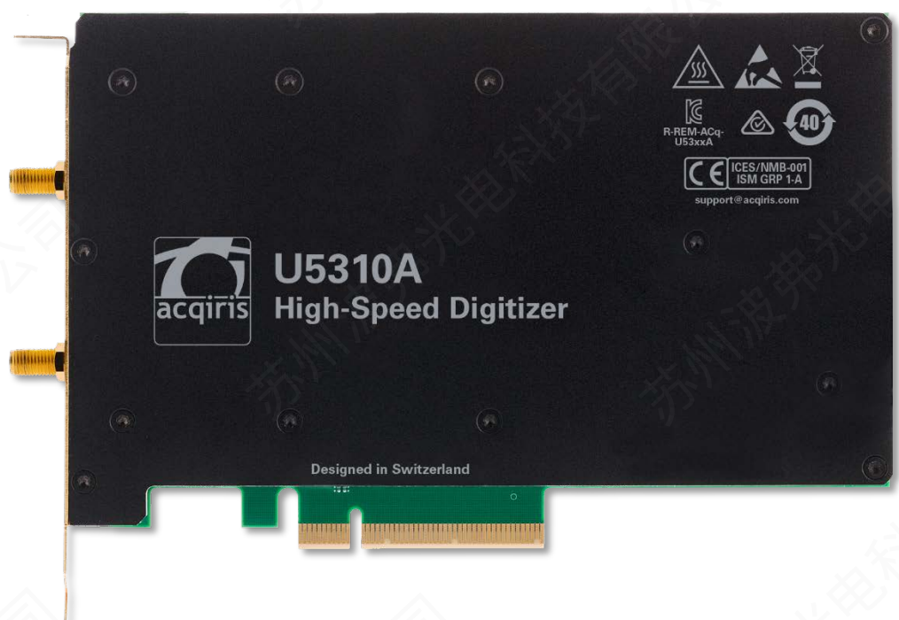
Figure 4. The Acqiris U5310A PCIe 10-bit ADC card with on-board processing offers a small size for easy integration.
