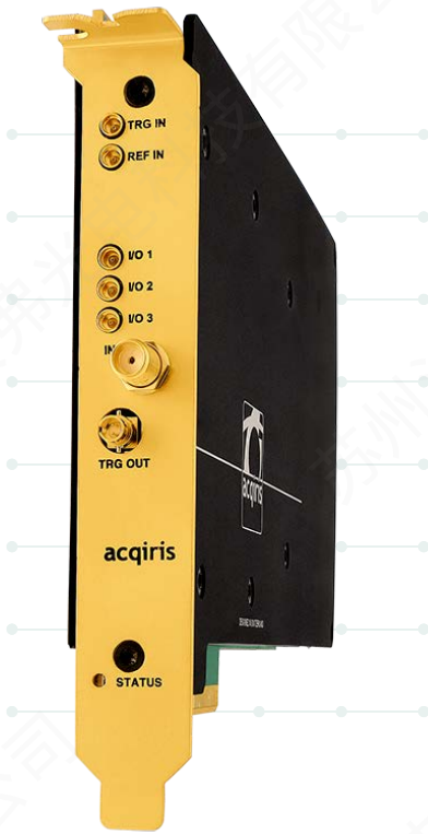
Figure 6. The SA248P is a fully shielded PCIe Card maximizing both ESD and EMI protection.
